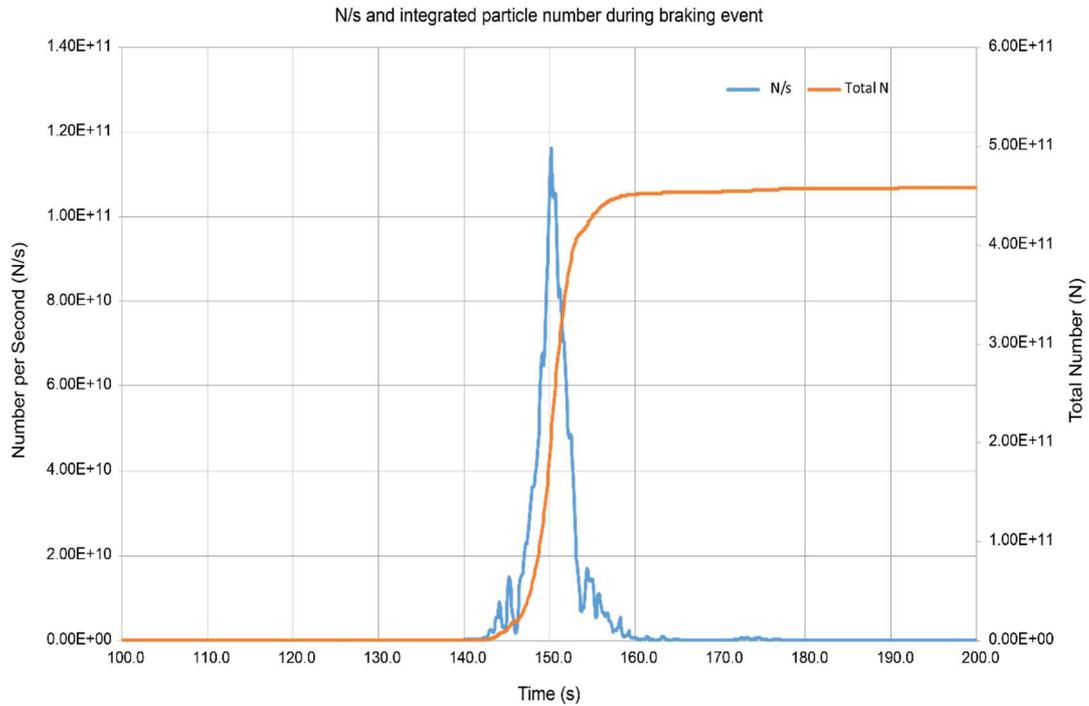
Historically, monitoring of particles from brakes has focused above 1 micron. The DMS500 was also operated on the 5 – 2,500 nm range to allow investigation over an increased size range.
