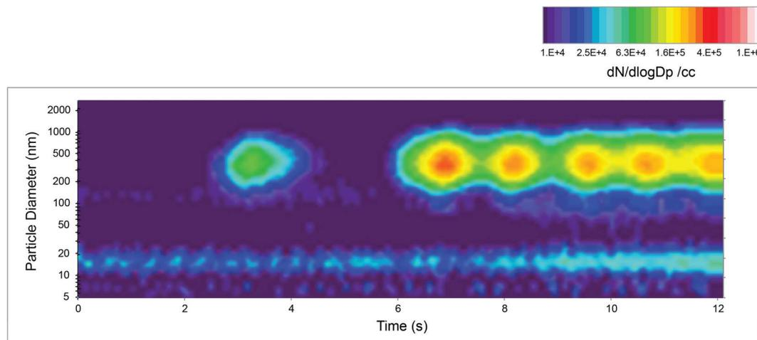
The above data suggest that for the DMS500 measurements on this brake system, a 5 nm – 1,000 nm measurement range is appropriate, since no particles were detected between 1,000 – 2,500 nm.
