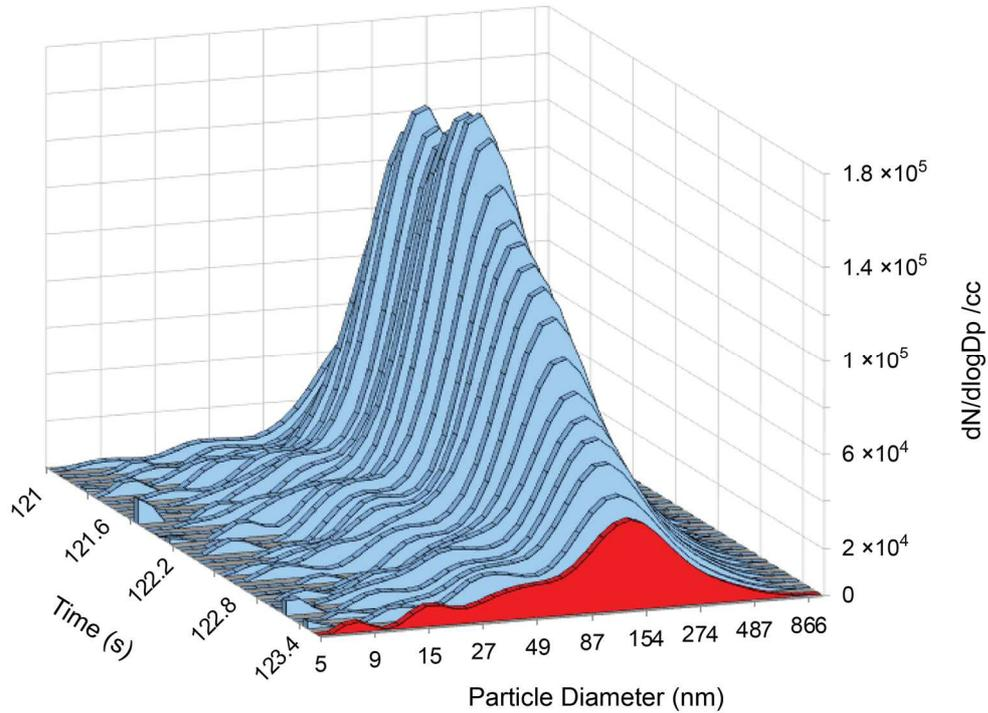
During repeated similar brake applications, the emission of particles increases with each application- it is presumed that this follows a trend with disc temperature.
