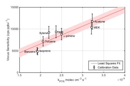
Figure 1 Sensitivity of Vocus PTR-TOF as a function of analyte proton transfer reaction rate constants,  $k_{PTR}$ . The linear relationship enables the calculation of sensitivity for compounds having known  $k_{PTR}$  without use of a standard.
