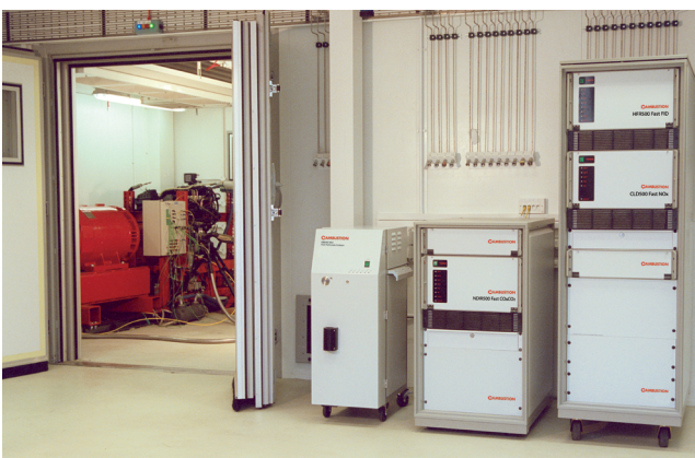
DMS500 shown with other ultra-fast Combustion analyzers (HC, NO x , CO & CO 2 )
