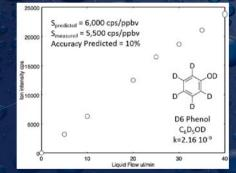
Vocus sensitivity for many compounds can can be estimated using published reaction rate coefficients.
