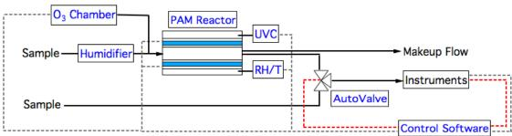
Typical setup for measurements incorporating PAM reactor. Control software facilitates datalogging at 1 Hz and automated control with event sequencing for unattended operation (dashed grey = analog input/output; dashed red = digital input/output)
