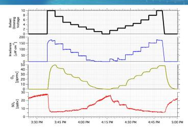
Time series from an example OH exposure calibration experiment using  $SO_2$  as a reactive tracer species. The dimming voltage applied to UV lamp ballasts is stepped from 0-10 VDC, which varies the UV irradiance and the ozone mixing ratio in the PAM chamber.
