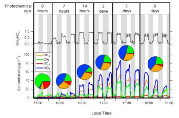
Example measurements obtained with a PAM reactor. Secondary ammonium, sulfate, organic, and nitrate aerosols are generated from OH oxidation of gas-phase motor vehicle emissions inside the Fort Pitt Tunnel in Pittsburgh, Pennsylvania, USA (<u>Tkacik</u> et al., Environ Sci. <u>Technol</u>, 2014). Shaded periods are when the tunnel air bypassed the PAM reactor.
