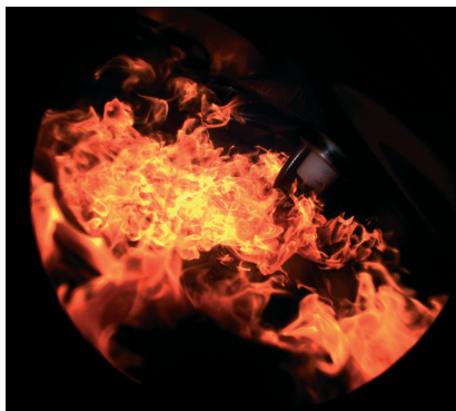
Pool fire on cold piston
