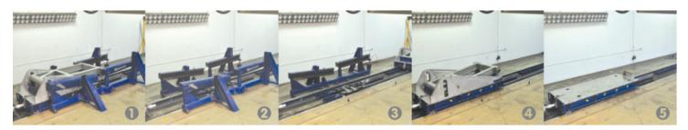
Removing the onboard equipment leaves a flat floor with full access to the sled system for uncompromised non-pitch testing and unobstructed camera views. There is no fixed equipment blocking access to the sled, and no complicated, expensive changes are required to the system.
