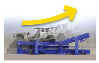
Adding pitch simulation to sled test systems for full frontal impact testing can improve the correlation of occupant injury performance between sled tests and barrier tests, providing engineers with better design data resulting in better engineering and safer vehicles.
