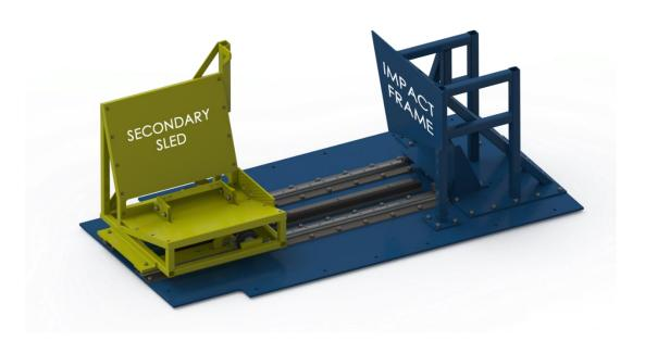
Enables testing to new NHTSA Child Restraint System (CRS) Side Impact regulation (2014 amendment of FMVSS 213)
