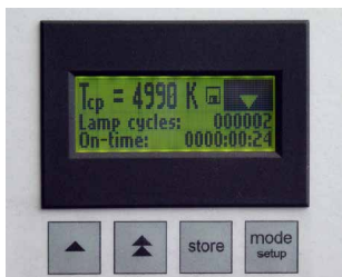
Left: Display and control of color temperature
