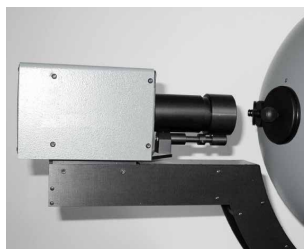
Right: Directional light source, color temperature regulated to standard illuminant A
