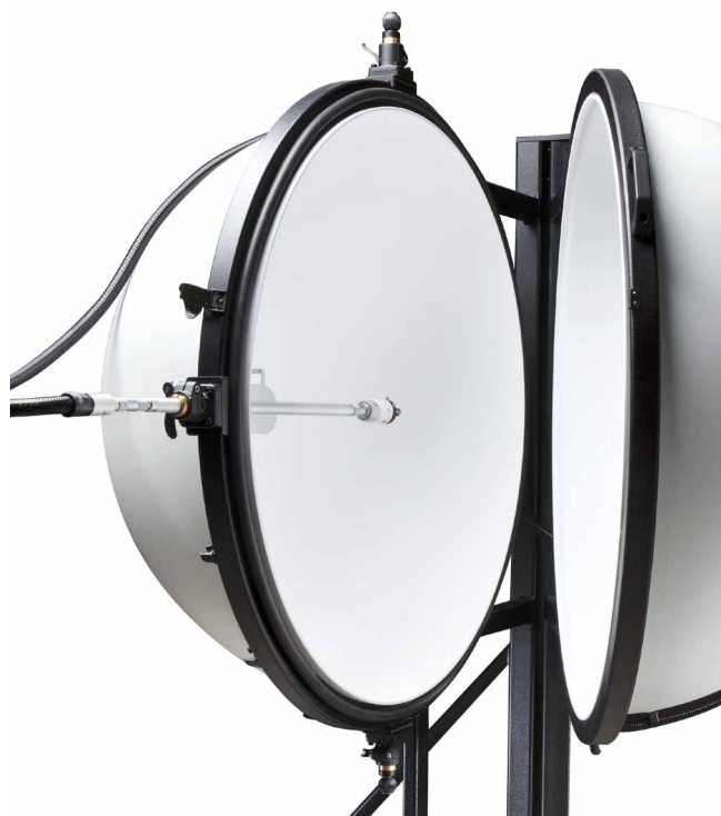
Internal view: three burning positions, up-side, down-side (vertical), front-side (horizontal)
