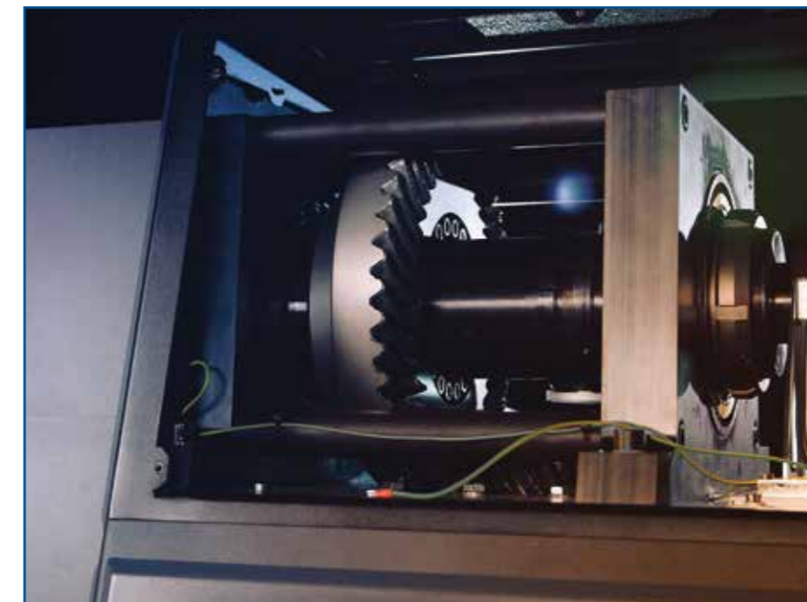
Gearwheel of the V-axis of the AMS 5000. Travel range of the H-axis is ± 200°, of the V-axis ± 100°, at an angle sensor resolution of 0.01°
