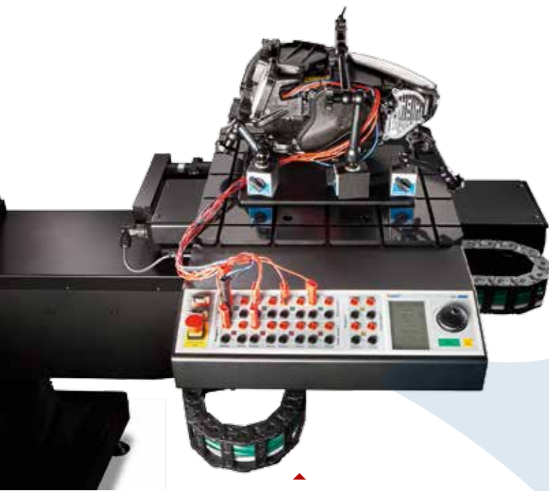
▲ Sample stage with lamp multiplexer
